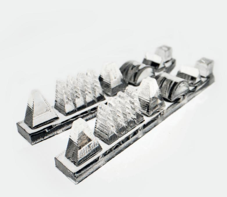
Top: 3D inkjet printed waveguide for a LED matrix.
